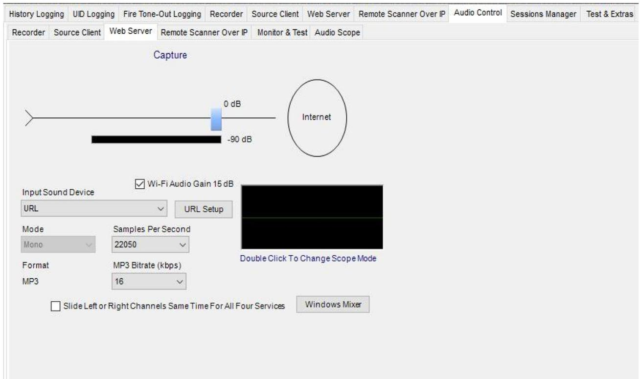
NOTE: This will allow the audio coming from the BCD536HP to be sent with your stream (feed) without having to use any physical audio cable connection between the scanner and your PC. The audio quality using the Wi-Fi method above is superior.
